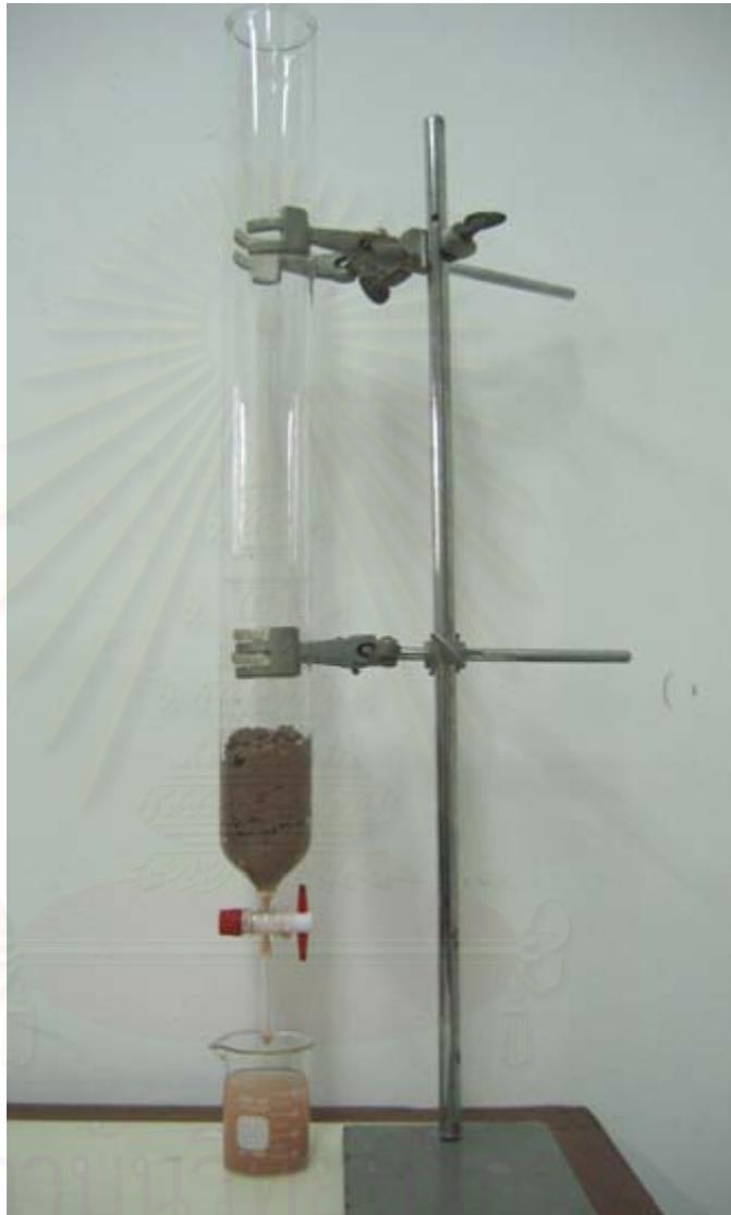
Figure 3.10 Application with the soil mining wastes studied in column with 50 mm of diameter x 500 mm long.
