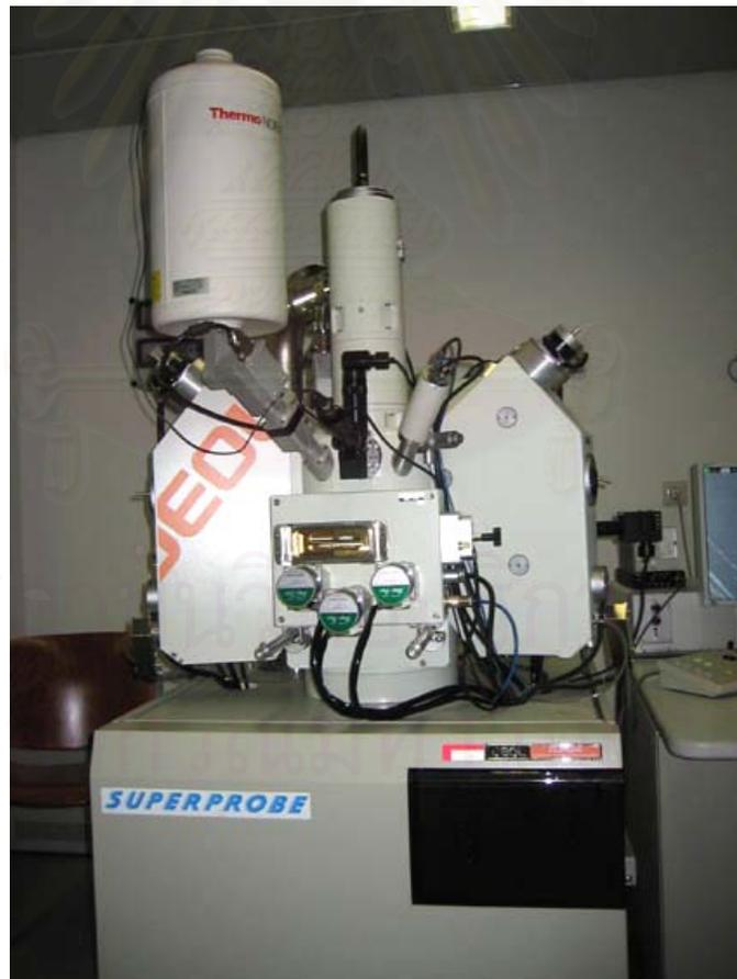
**Figure 3.8** Electron Probe Micro Analyzer (EPMA) used for analyzing the chemical composition on the pyrite surface (Available from: [www.hardcoatings.ac.at](http://www.hardcoatings.ac.at)).
