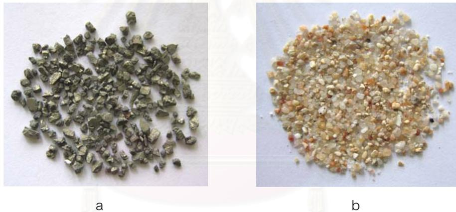
Figure 3.1 Pyrite samples (425 - 850  $\mu\text{m}$ ) and sand (1 - 2 mm) before coating.
