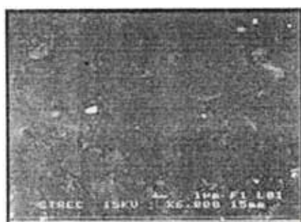
Vulcanized NR before UV exposure
