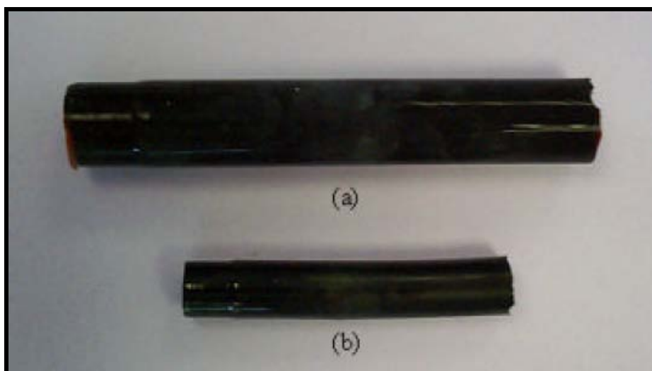
Fig. 3 Effect of the pyrolysis on a of resorcinol-formaldehyde aerogel
