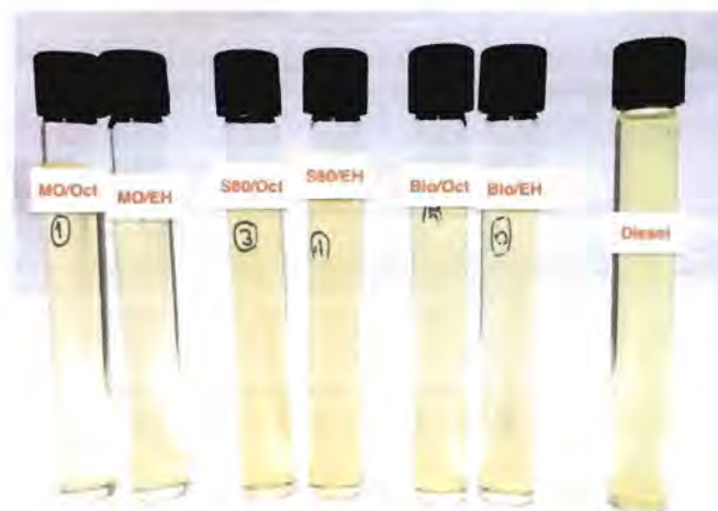
Figure 18 Turbidity of all of palm oil/diesel blend with 20 vol.% of ethanol systems after held at room temperature ( 25\pm 2^\circ\text{C} ) for 48 hours.
