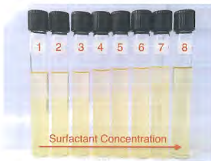
Figure 16 Phase behavior and turbidity varying surfactant concentration of methyl oleate/1-octanol with a palm oil/diesel blends at a ratio of 1:1 (v/v) and ethanol.
