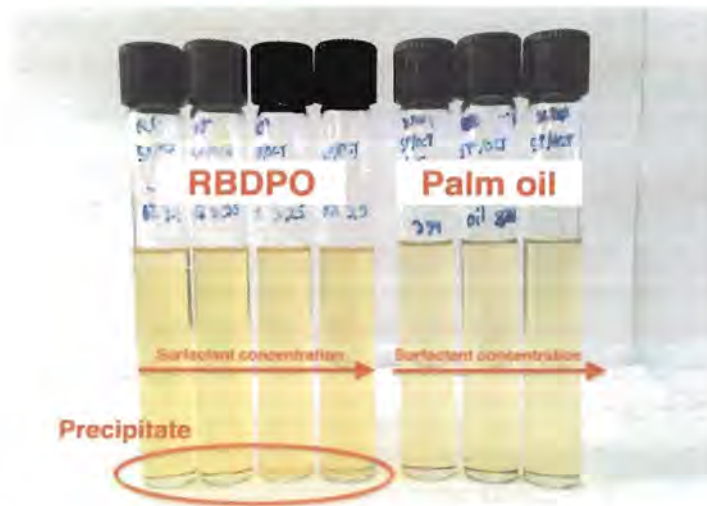
Figure 17 Phase behavior and turbidity comparison of Span 80/1-octanol system in RBDPO/diesel blend and palm oil/diesel blend at a ratio of 1:1 (v/v) with ethanol.
